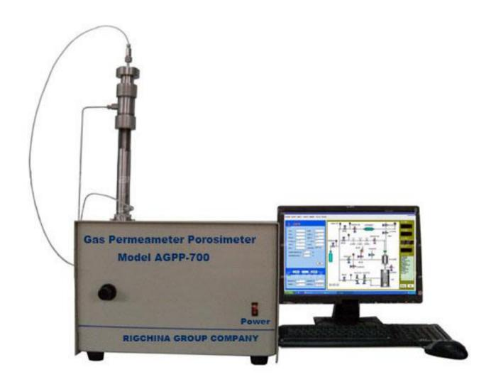
The AGPP-700 is an automatic and highly accurate system for determining rock properties such as permeability, Klinkenberg permeability, pore volume, porosity and grain volume at overburden pressure. The system uses an unsteady state pulse decay technique for the permeability measurement.
