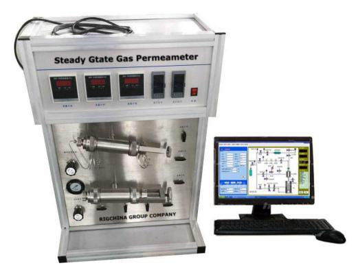
The Automatic Gas Permeameter is an automatic and highly accurate system for determining rock properties such as permeability, Klinkenberg permeability, pore volume, porosity and grain volume at overburden pressure. The system uses an unsteady state pulse decay technique for the permeability measurement.
